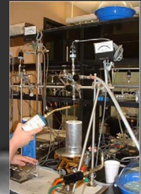
FIG. 4 Diagram of a Mass Spectrometer FIG. 5 (left) Sample funnel. FIG. 6 (above) Gas treatment line (purifies \text{CO}_2 for testing) FIG. 7 (right) Flame sealing \text{CO}_2 sample for analysis
