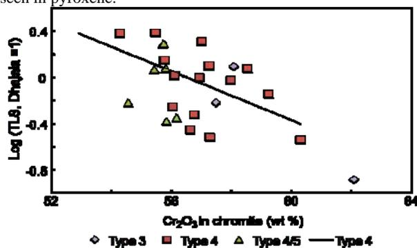
Figure 3 – TL Sensitivity is compared with the changing  $Cr_2O_3$  content in chromite.
