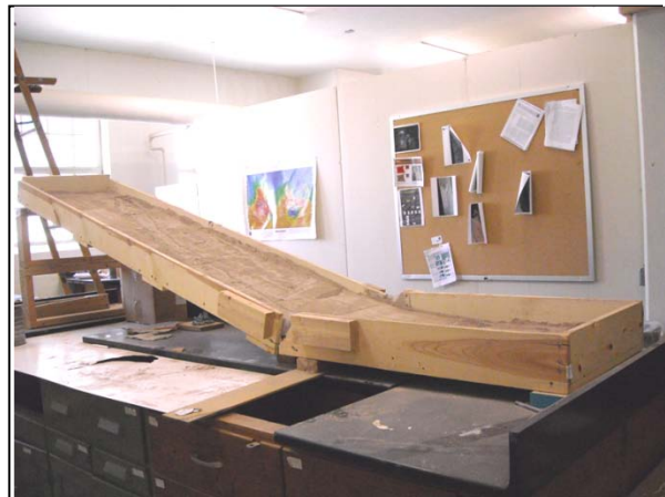
Figure 1: One of the wooden flumes that was constructed to study the streak-like features in the simulations.
