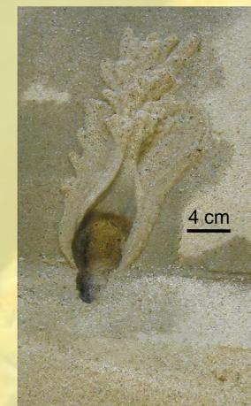
Fig. 8: Gully morphology created using  $\sim 1500 \text{ mL}$  of solution with a somewhat long and narrow apron.
