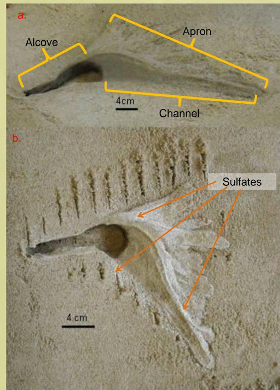
Fig. 3: a. Gully morphology created using  $\sim 736 \text{ mL}$  of solution. b. Same gully left to dry for 48 hours resulting in the formation of sulfates (white material) on the surface of the apron.
