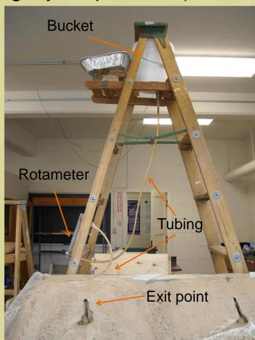
Fig. 2: Experimental set up used to create gullies.
