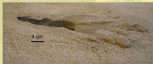
Fig. 4: Gully morphology created using  $\sim 947 \text{ mL}$  of solution.
