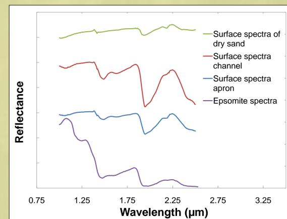
Fig. 5: FTIR surface spectra plot showing epsomite present on the surface of gully channel and apron.
