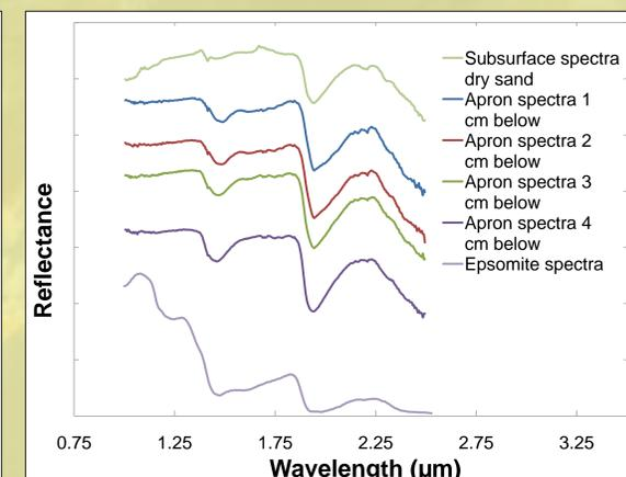
Fig. 6: FTIR subsurface spectra plot of the apron showing epsomite is detected.
