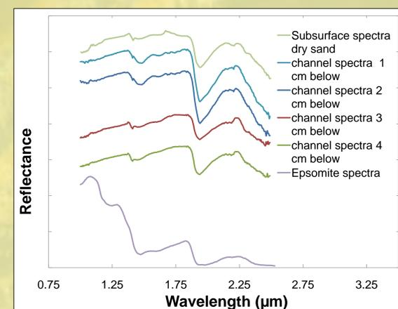
Fig. 7: FTIR subsurface spectra plot of the channel showing epsomite detected down to 2 cm.
