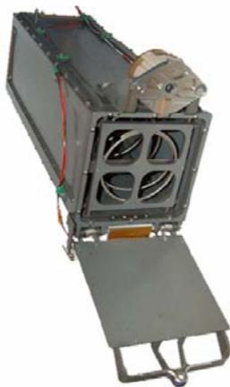
**Figure 2: PPod Launcher Ref. 1**
