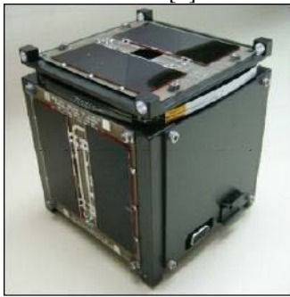
Figure 1: Basic 1U CubeSat [3]
