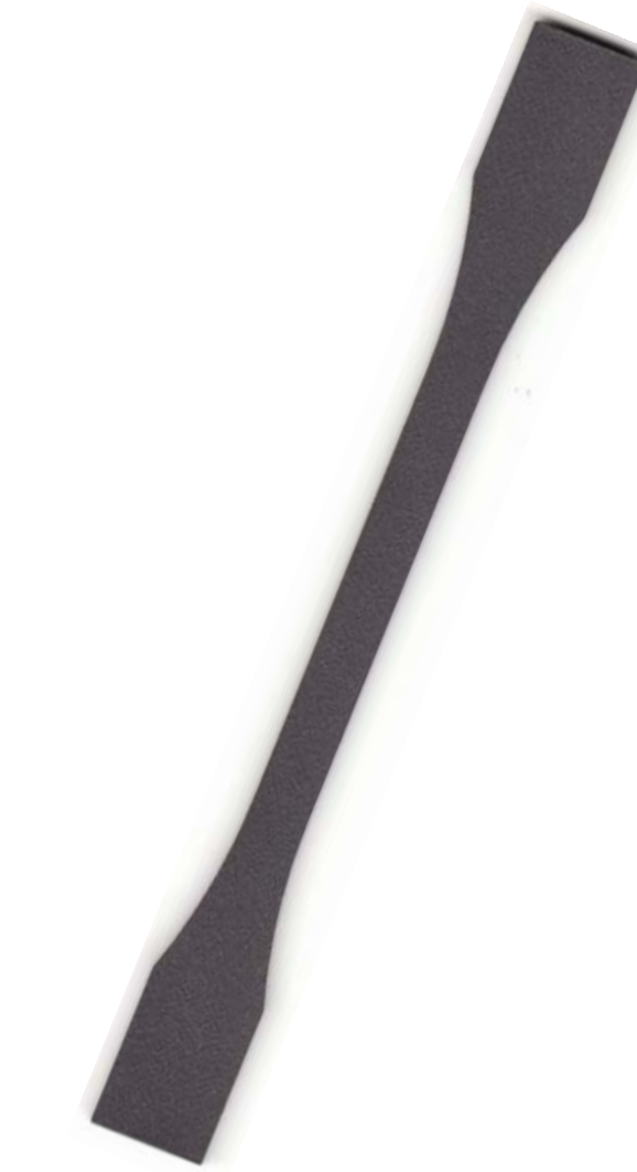
Figure 9: ISO 527-Flat “Dog-bone” Standard
