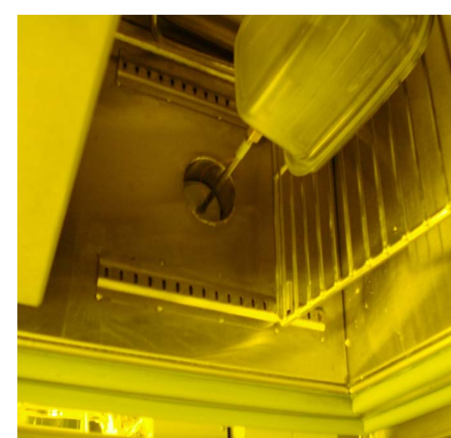
Figure 6: Contained Test Cube Attached to Stem in MCBH Temperature Chamber
