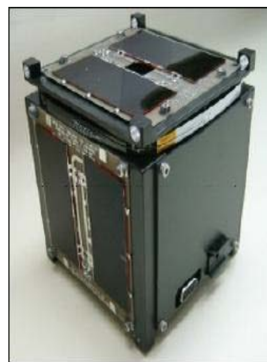
Figure 1: Basic 1U CubeSat
