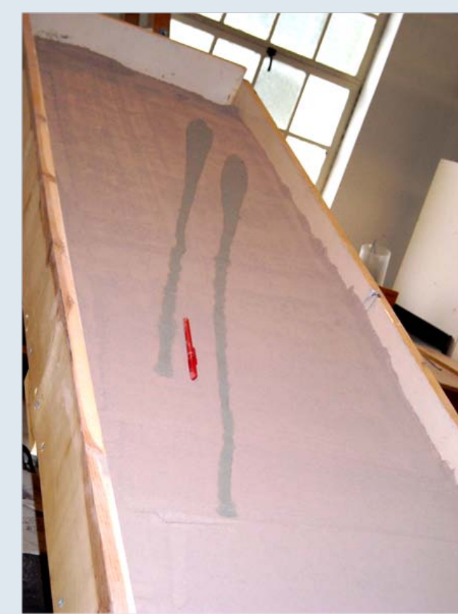
Figure 4: These simulations were run at room temperature using a solution of viscosity 0.724 Pa s on MMS at a 20 ° slope angle.
