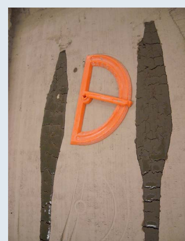
Figure 6: This simulation was obtained using a solution of viscosity 0.075 Pa s that was run at room temperature with a 10 ° inclination angle. The cracks here are especially visible.
