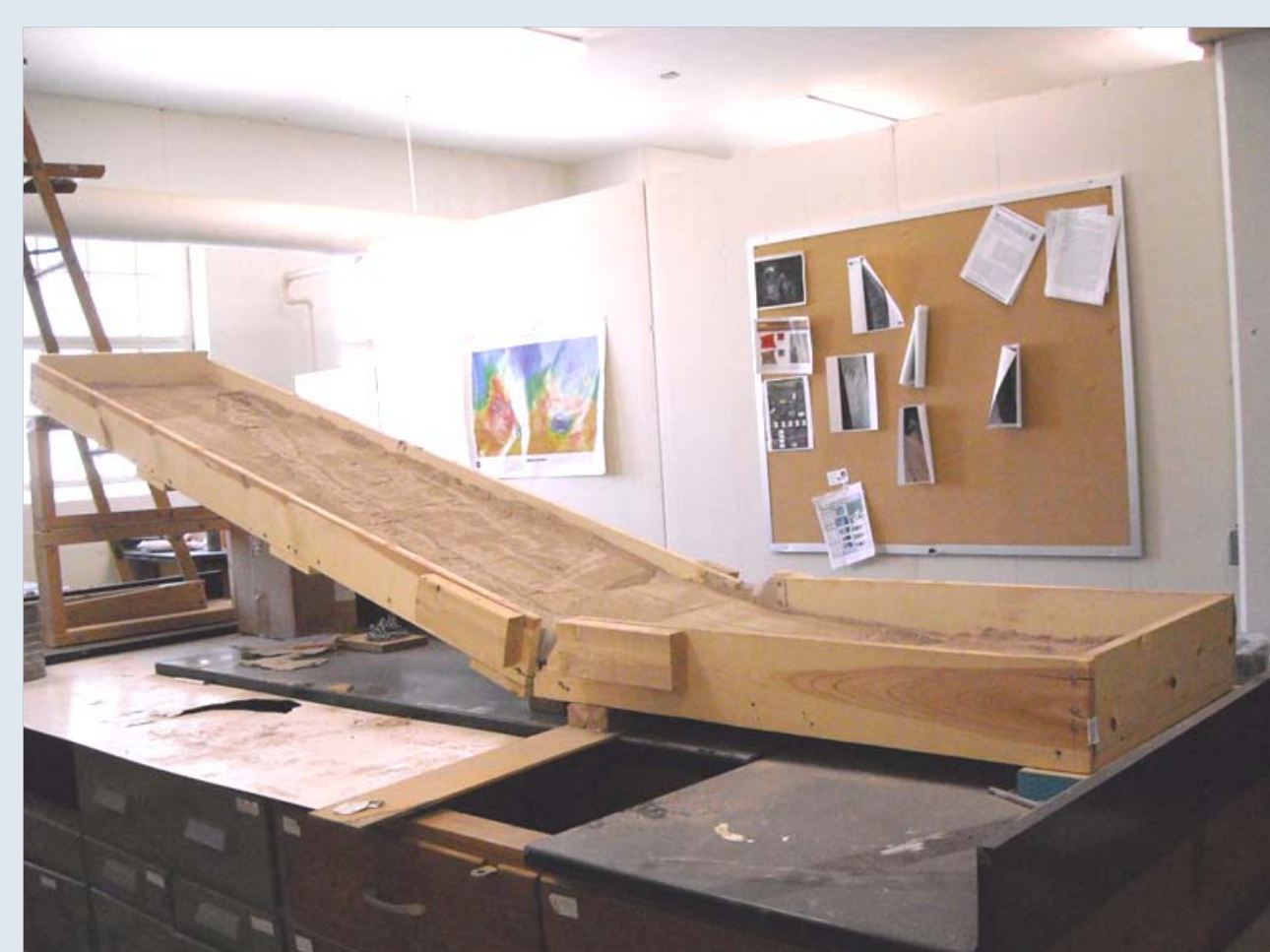
Figure 2: Simulations at room temperature are run in this flume filled with Mars Mojave Simulant, which consists of finely ground up basalt.
