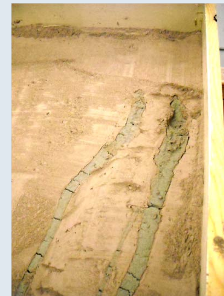
Figure 3: These simulations were run at room temperature using a solution of viscosity 0.021 Pa s on MMS at a 20 ° slope angle.
