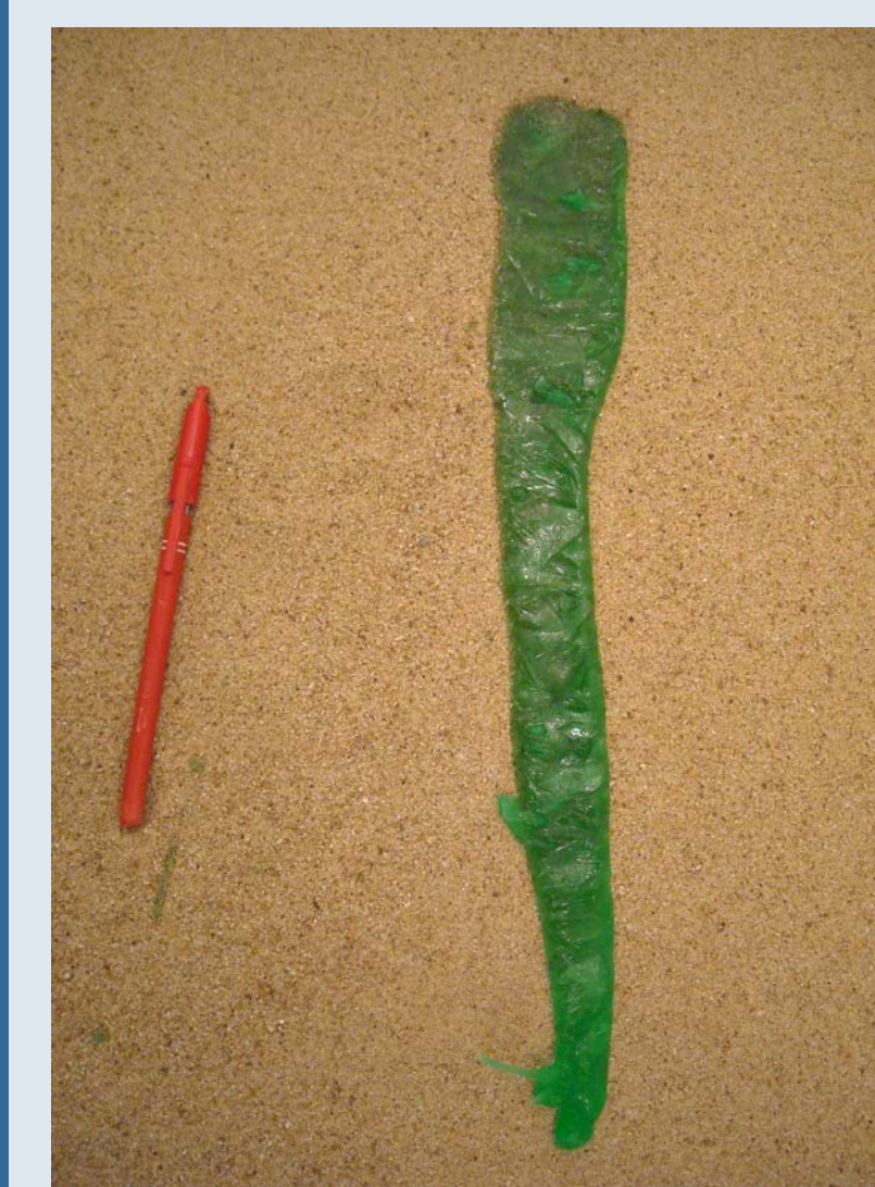
Figure 8: This simulation was run at -20 °C using a solution of viscosity ~ 1 Pa s on sand at a 20 ° slope angle.
