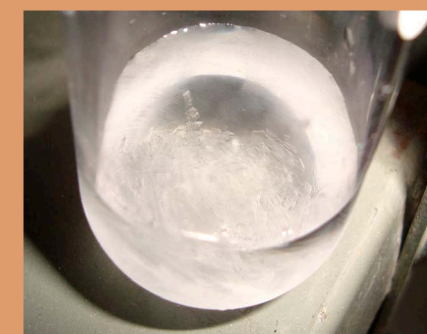
Figure 2. Crystallized MgCl 2 at -22°C
