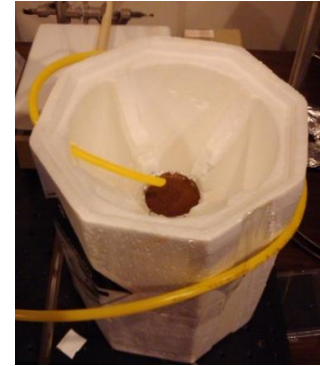
Figure 1: Improved Styrofoam chamber used to take spectra. The sample is in the center surrounded by dry ice. The yellow tube allows nitrogen to flow over sample.
