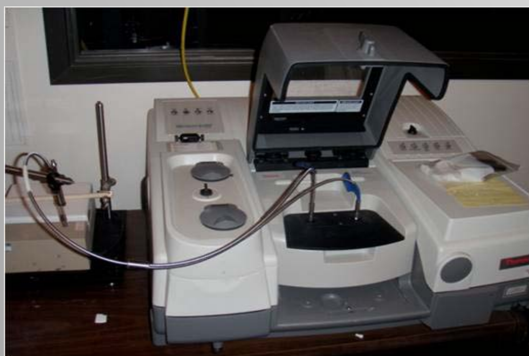
FTIR spectrometer used for the collection of all spectra. Shown with Smart NIR Probe accessory and the fiber optic probe attached.
