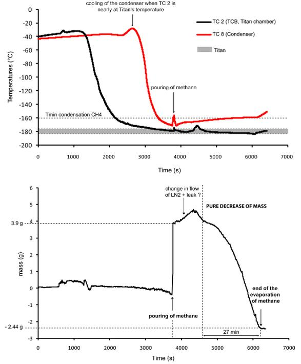
Figure 1: Temperature and mass recordings versus time. The condenser is cooled to synthesize liquid methane from gas once Titan's temperatures are almost reached in the TCB under Titan's pressure. The mass sharply increases when the liquids are poured in the Petri dish and then decreases.
