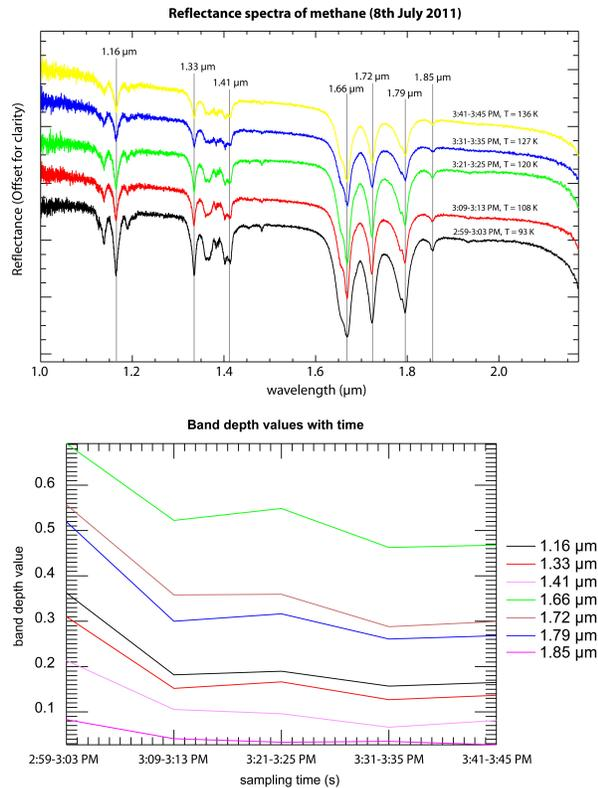
Figure 2: Top: example of FTIR spectra of liquid methane acquired during a run at Titan's pressure. Bottom: computed band depths values from the liquid methane spectra.
