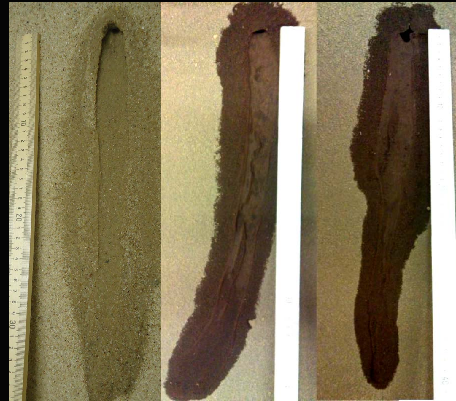
Fig. 3: Comparing resultant gullies of preliminary sand tests (left) to two consecutive runs in JSC Mars-1 (right) to illustrate the difference in uniformity when working with smaller particle sizes
