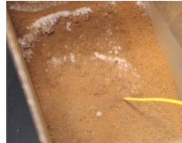
Fig. 5. Still image of a large collapse that occurred at 34° slope.
