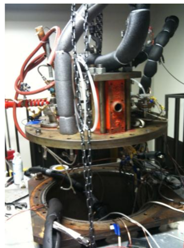
Figure 1. Photograph of the outside of the Titan chamber, with the top of the chamber suspended in the air.
