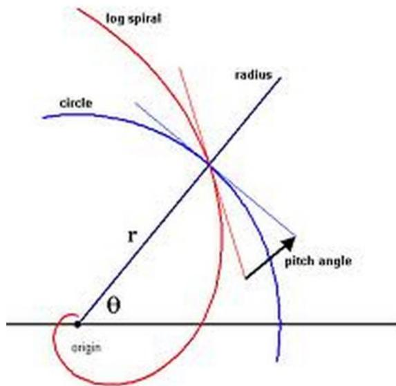
FIG 1. Pitch angle decomposition by constructing a circle (blue) intersecting a logarithmic spiral (red) at some radius  $r$ . If lines are drawn tangent to the circle and the spiral at the intersecting point, then the pitch angle is the angle between the two tangent lines. A circle would have a pitch angle of 0 degrees and a radial line would have a pitch angle of 180 degrees.
