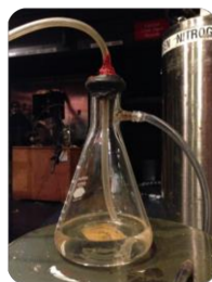
Figure 2. CH 3 CN saturation apparatus. N 2 gas bubbles in from the top and the gas mixture flows out through the side to the chamber.
